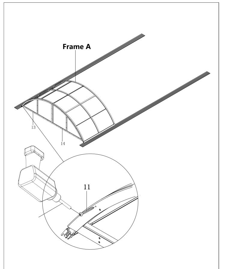
Drill Ø4.8 holes first in the Frame A along the current hole and then Mount the half door (13/14)to the Frame A with the screw ST 5.5\*50(item 11)
