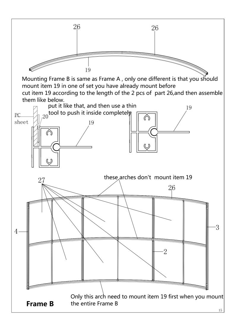
The mounting steps for Frame B/Fram C and FrameD is same. Don't forget to mount item 19 first in one of the set when you mount Frame C and D.
