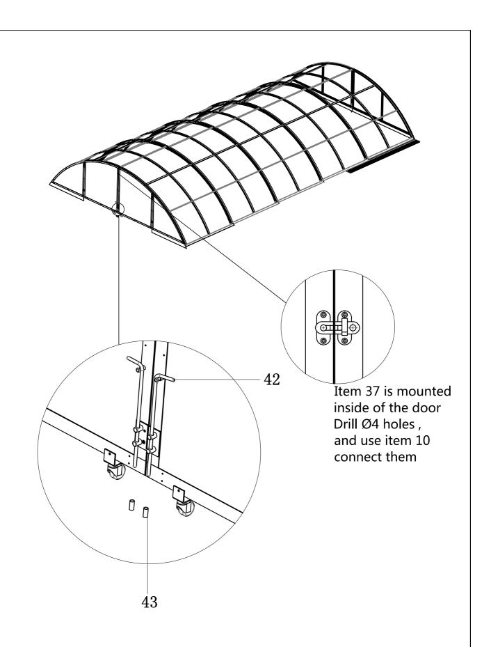
These parts are mounted outside of the door. You need to cut the dust cloth, so that the wheels can be used
