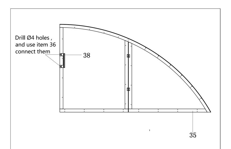
Drill Ø4.8 holes first in the Frame E along the current hole and then Mount the half door (34)to the Frame E with the screw ST 5.5\*50(item 11)
