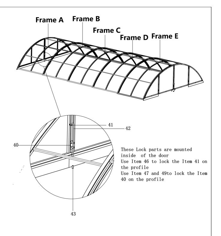
Item 43 is mounted on the ground, you need to drill a hole, and then put 43 in it, 43 and 42 must be in a line, so that 42 can put in 43 to lock the door.
