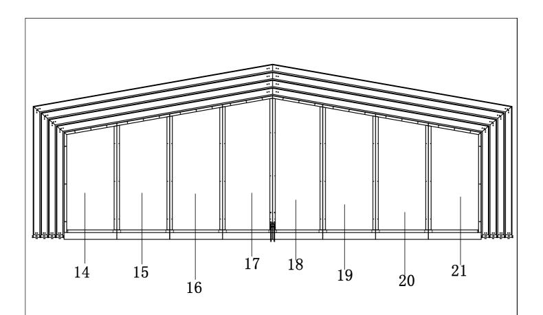
Item 14/15/16/17/18/19/20/21 is mounted on the section 1, You first drill Ø4.8 hole according to the Ø6 hole in these windows, and then use item 62(5.5\*50) to connect them in the section 1
