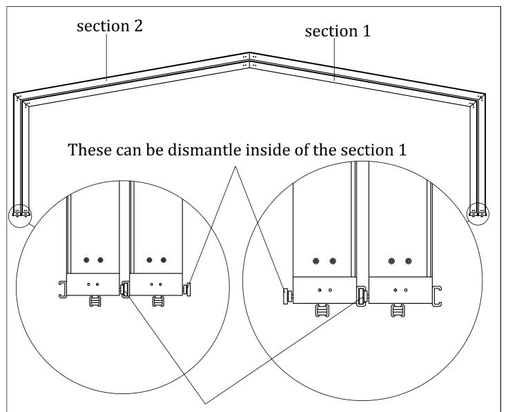
If you think use two side rails is a little difficult for mounting, you can dismantle the wheels on the item 11( side wheels). Use one side is enough for controling the direction.
