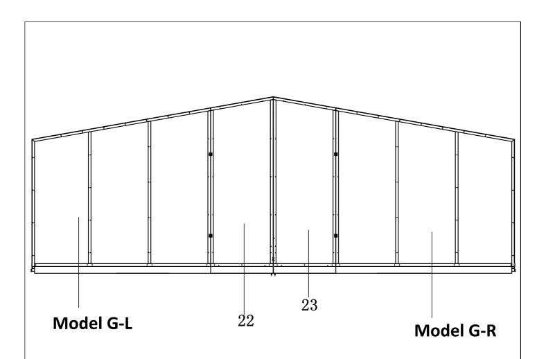
First mount the Model G-L and Model G-R on the section 5 (biggest section) with the item 62. And then you mount item item 22 on the left with the hinge (46)/47 and 48 together.
